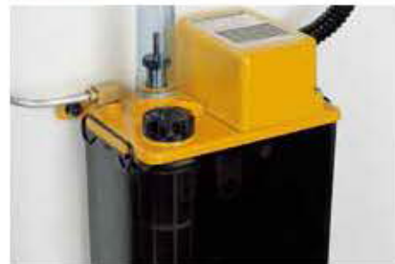
INTEGRATED AUTO LUBRICATING SYSTEM FOR ALL SLIDEWAYS 滑道採用自動潤滑器
