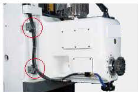
The Y, Z axis slideways are secured by compressed air, max. pressure of 1500 kg/cm 2 , to avoid table movement while heavy cutting, thereby ensuring workpiece accuracy (For VH450, only Y axis is applicable for this function) (Opt.) Y, Z 兩軸滑道採用空壓裝置固緊，最大固鎖力可達1500公斤/平方公分，即使進行重銑削工作，工作檯面無偏差滑動，確保工件成品精密度 (VH450只有Y軸可裝) (選配)。
