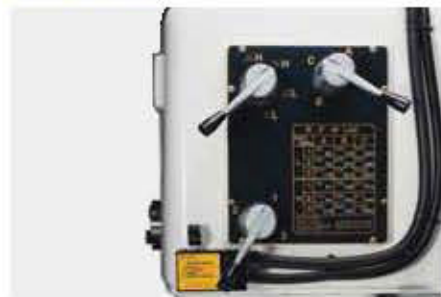
45- 1500 RPM 18 SPEED CHANGE 45- 1500 RPM 18段變速
