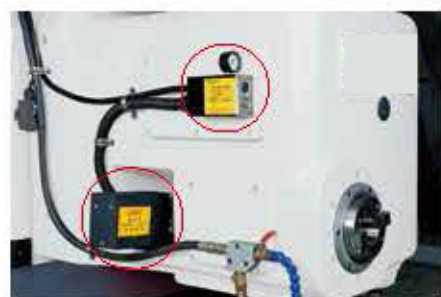
Air power draw bar (Vertical and horizontal spindle, 450, 550, 650, 780) 氣動鎖刀裝置(立式及橫式主軸，450, 550, 650, 780)
